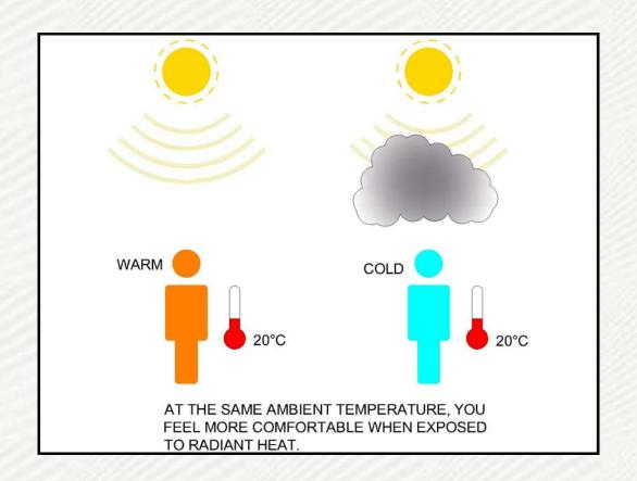
Like the Sun's rays, radiant heat moves in straight lines, warming all objects in its path. These objects in turn become heat radiators, giving off their own gentle heat thus preventing building occupants losing warmth to cold objects such as walls, floors, tables, chairs, etc. Air is transparent to the transfer of energy, which occurs directly from warmer to cooler objects.
